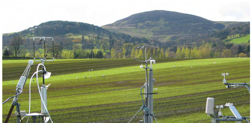
Measuring nitrogen emissions from slurry spreading at UKCEH's Edinburgh research site
