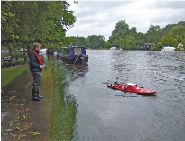
**Plate 7:** Flow measurement using an Acoustic Doppler Current Profiler in the river Thames (July 2007)
