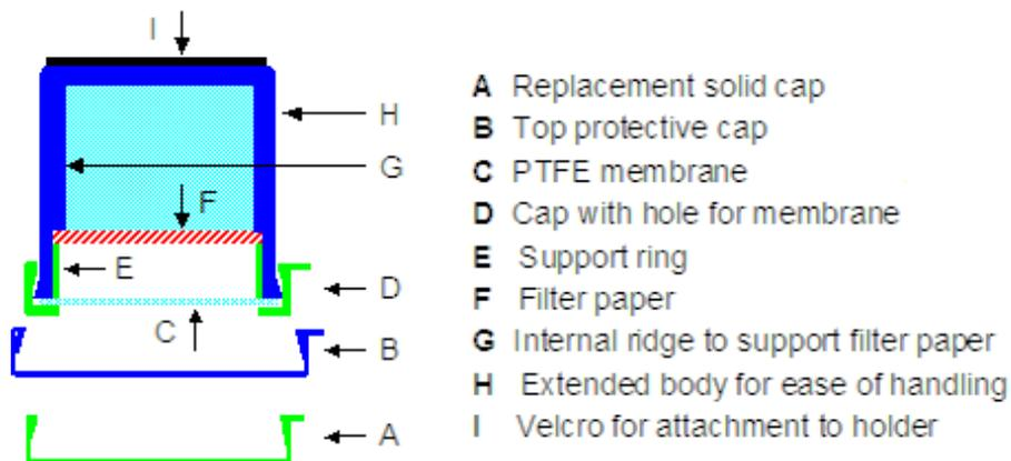
**Figure 1:** Outline diagram of a single CEH ALPHA® Sampler
