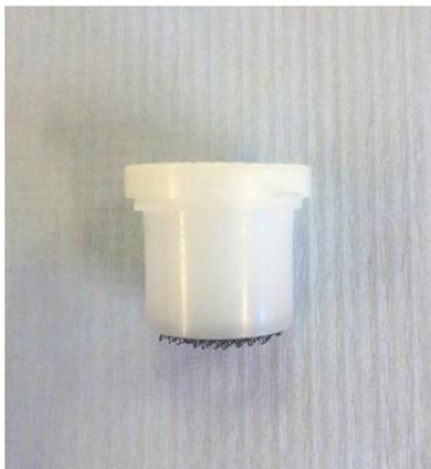
**Figure 2:** Assembled CEH ALPHA® sampler.
