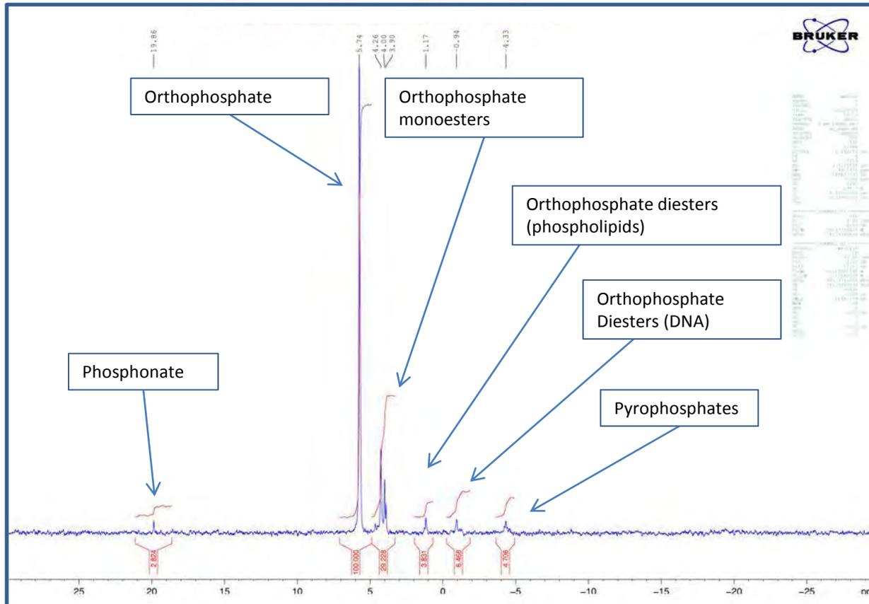
Nuclear magnetic resonance ( $^{31}\text{P}$ -NMR) spectroscopy showing different compounds present in the effluent of a septic tank in the Loch Leven Catchment, Scotland, UK. Based on Cade-Menun 2010
