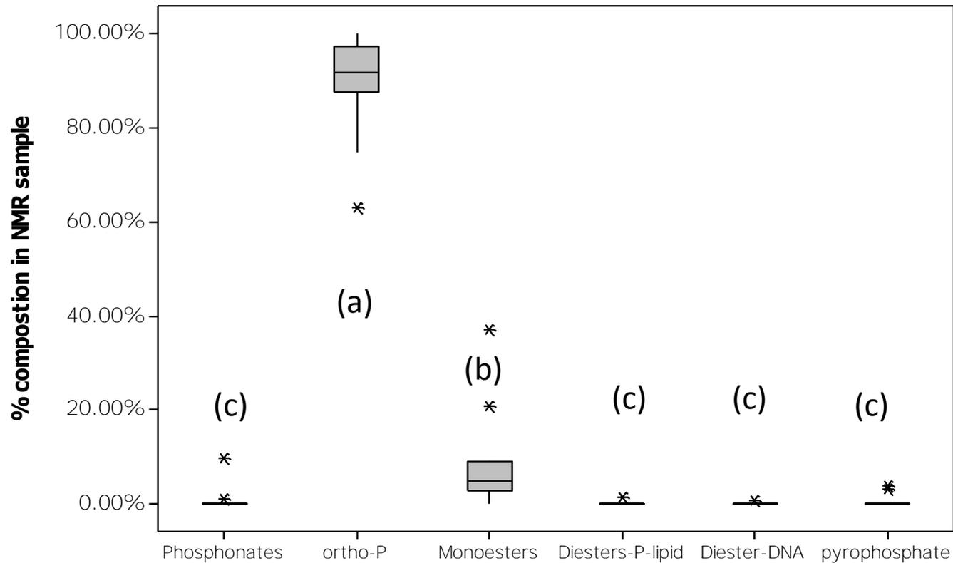
NMR samples contained an average 81.9% orthophosphate and 8.1% orthophosphate monoesters, with trace phosphonate, orthophosphate diesters and pyrophosphonates.
