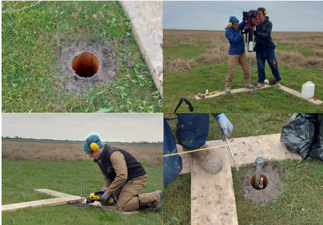
Setting the SET in with postcrete (Left). Installed SET base (Right).
