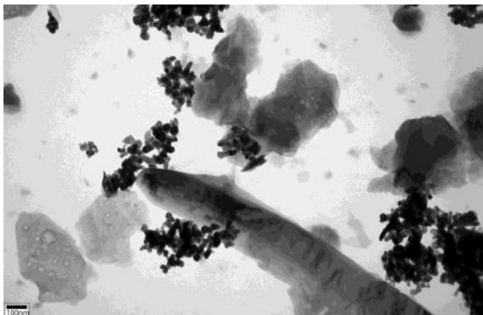
ZnO ENP agglomerates bound to dissolved organic matter in a soil extract.
