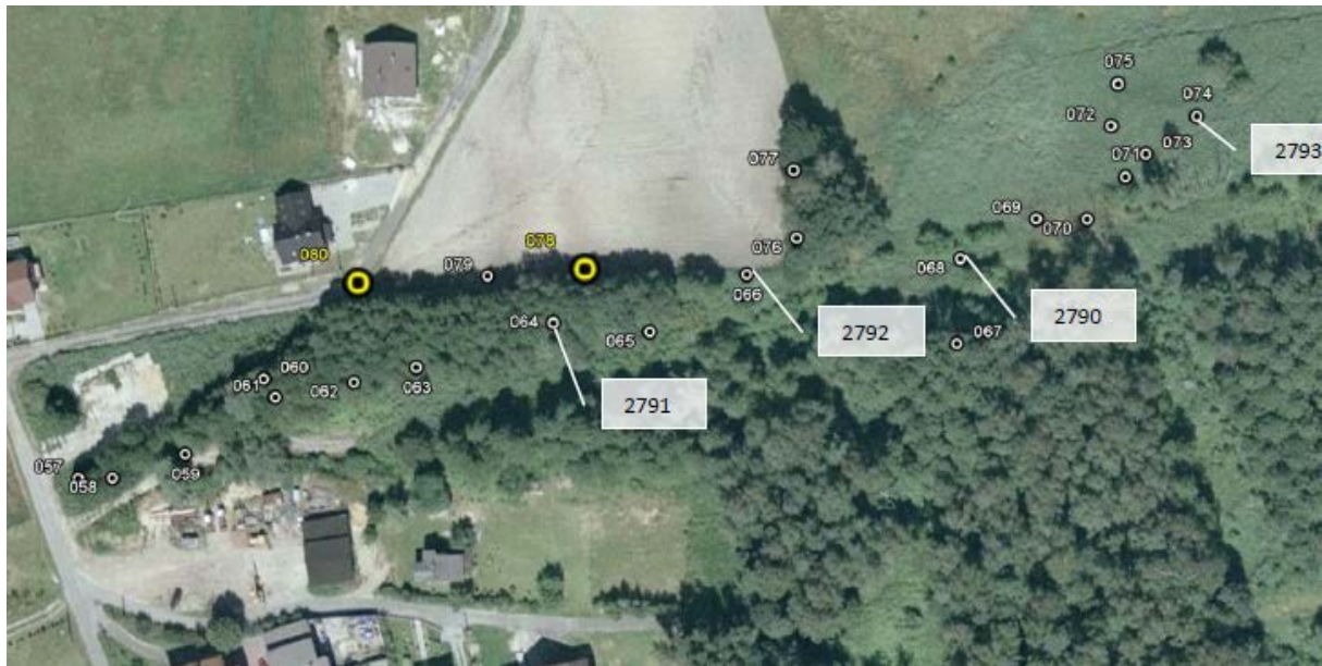
Figure 4.3.3.: Dose rate measurement and soil sampling points
