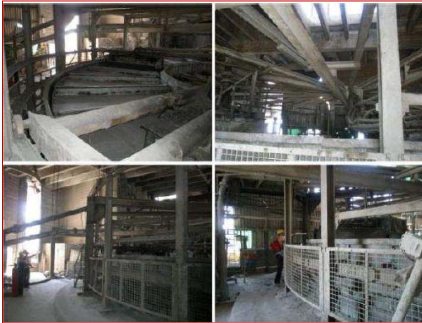
Figure 10 Filtration Unit of a Phosphoric Acid Plant where can be found radioactive particles
