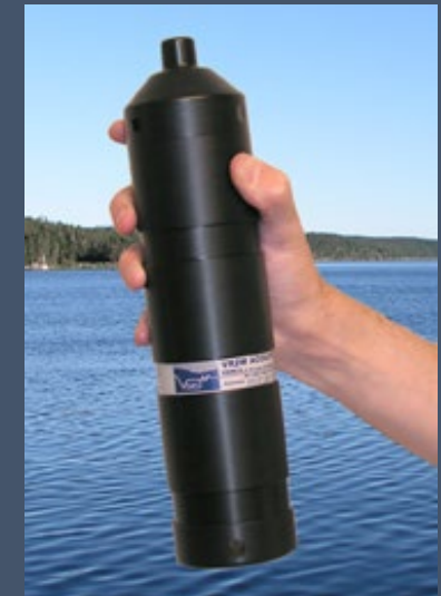
A fixed position acoustic listening station 2020s
