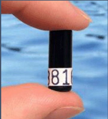
Tags: acoustic signal 69 kHz; coded to allow fish ID
