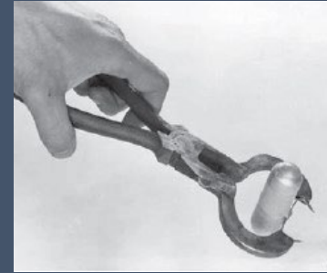
One of the first acoustic telemetry tags for fish ca 1956
