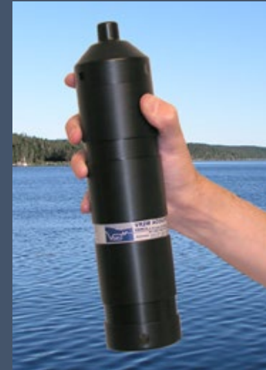
Receiver: detects and logs acoustic signal
