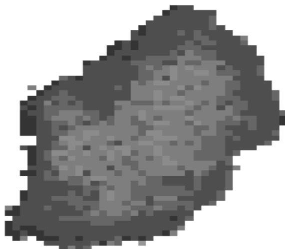
Figure 27. \mu -XANES imaging of a particle collected to the north of the Chernobyl reactor, released during the reactor fire. The particle has a UO_2 -core (U oxidation state 4) surrounded by an oxidised U_2O_5/U_3O_8 surface layer (U oxidation state 5)
