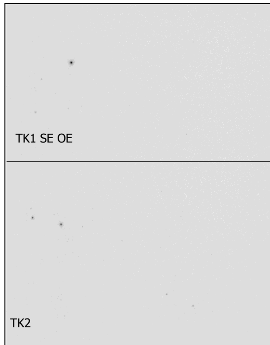
Figure 5. Digital phosphor imaging (autoradiography) of dried surface soils (1-5 cm) from the outer rim (south-east) of the Tel'kem 1 crater (upper) and from the outside (north) of the Tel'kem 2 crater (lower), respectively
